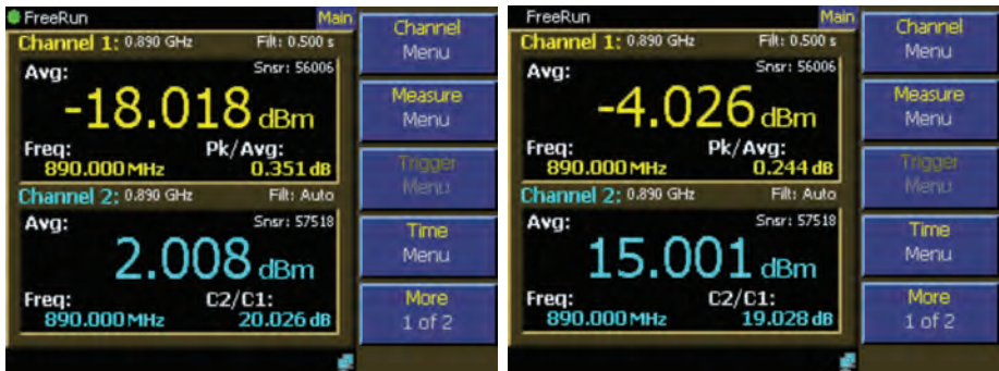
Figure 8.3.4. Two-Channel measurements showing amplifier gain (Channel 2 to Channel 1 ratio) dropping by 1dB
