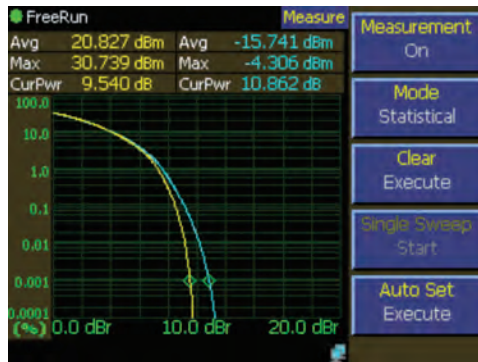
Figure 6.3.2. Dual CCDF: amplifier input on Channel 2 (blue, right), and amplifier output on Channel 1 (yellow, left)
